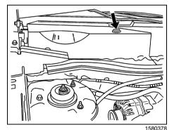
Remove the push pins from the rear of the passenger's side air inlet panel. It is located in the rear of the engine compartment on the passenger side of the vehicle.
